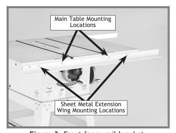
Figure 3. Front fence rail bracket.
